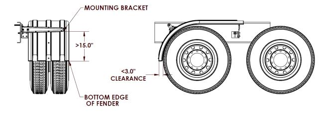
Figure 1 - Bracket Position and Clearance Example
