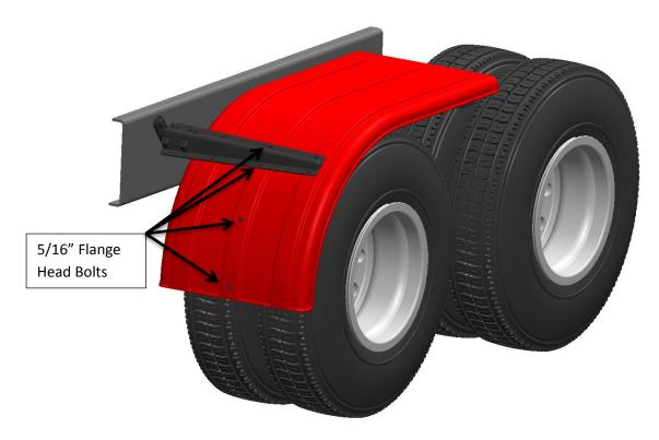
Figure 3 - View of 5/16" Fasteners (MIN 950)
