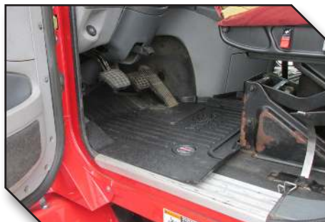
Figure 6 - Driver Mat Fit with OEM Seat Base
