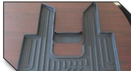
Figure 4 - Center Mat Trimmed for Set Back Gearshift
