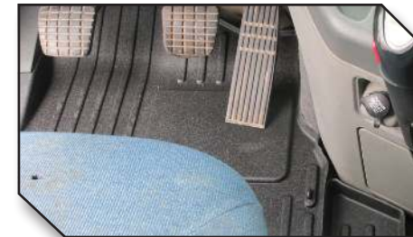
Figure 11 - Properly Installed Driver Mat and Hook
