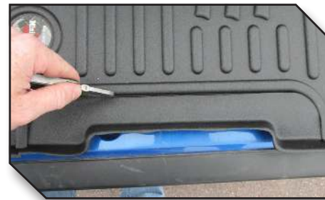
Figure 7 - Driver Mat Trim for Installation With Ezy Rider Seat or Aftermarket Seat.
