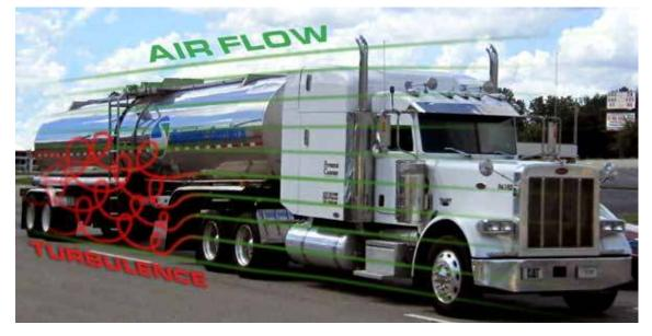
Air Products was curious about what would happen if they removed those fenders, so the fender was removed and the model trailer was put back into the wind tunnel. The result? A major reduction in aerodynamic drag. So Air Products decided to remove trailer fenders and instead put fenders on the rear drive axle of the tractor in order to reduce aerodynamic drag but still protect the tank trailer from road debris.
