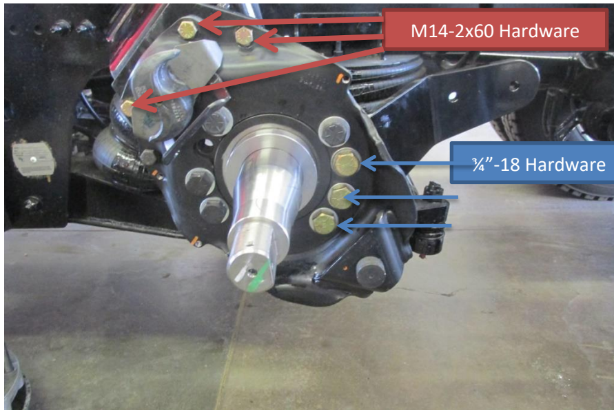
Figure 7 - View of Bolts & Brackets Installed
