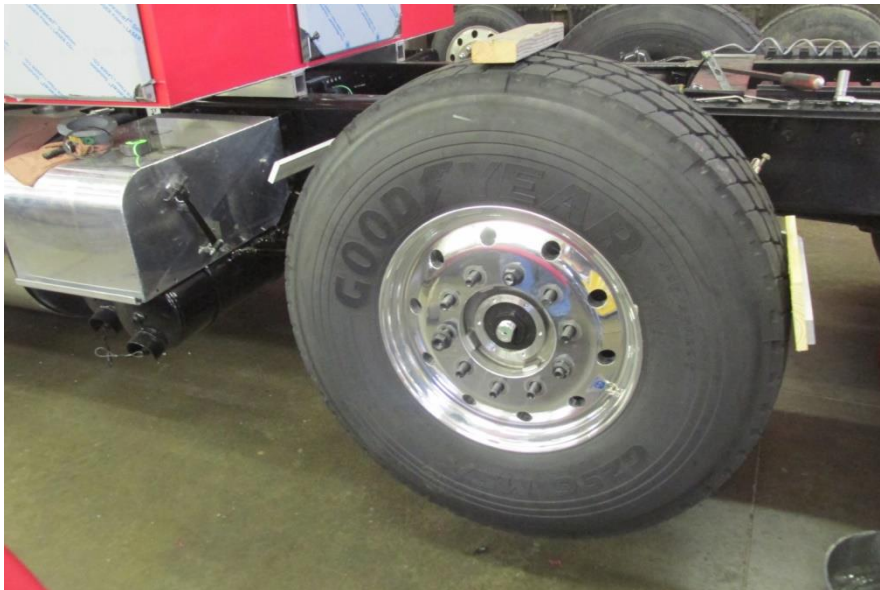
Figure 9 - Aluminum arms and wood blocks clamped in position
