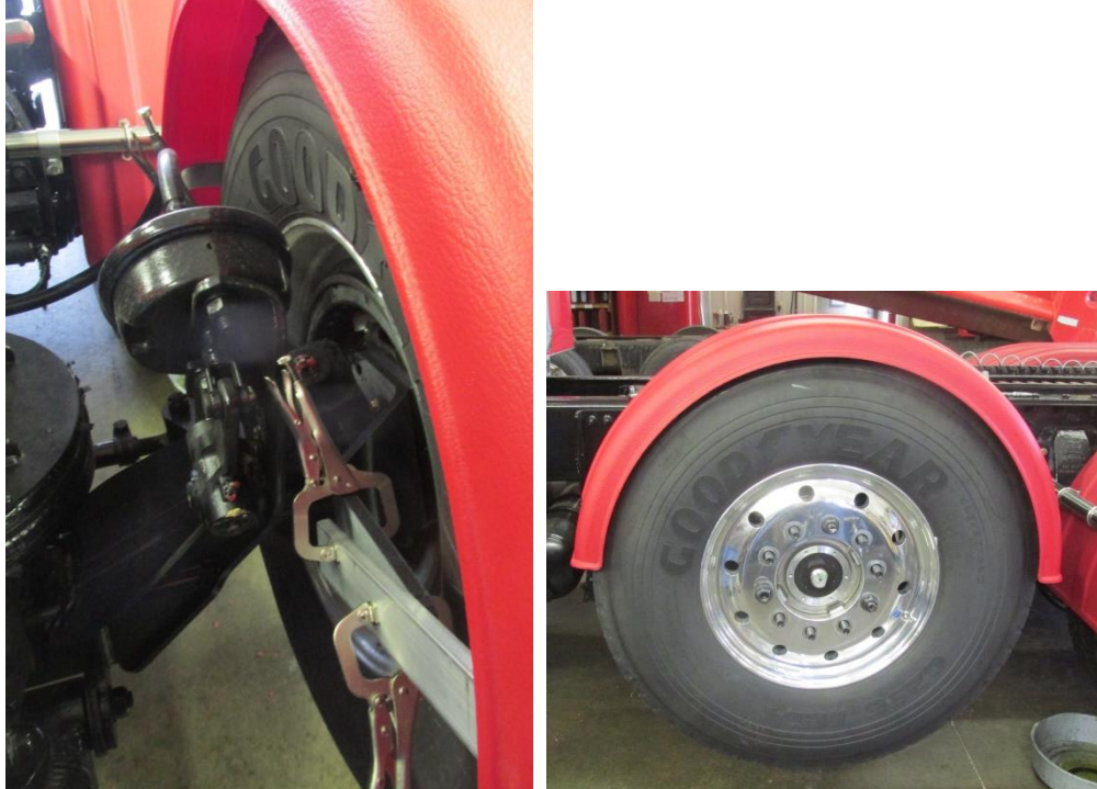
Figure 10 –Views of Fender Installed over Tire and Brackets
