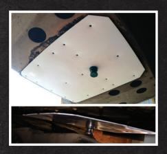
\*Warning: DO NOT use a Minimizer 5th Wheel Slick Plate, Trailer Slick Plate, Slick Disk, or a Mfg Low Lube 5th Whee Topplate in conjunction with one another. Doing so could cause a coupling failure. DO NOT INSTALL the Trailer Slick Plate if it extends past the front edge of the trailer or the upper bolster plate.
