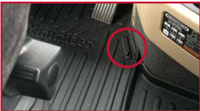
Figure 11 - Driver Mat Hook Installation
