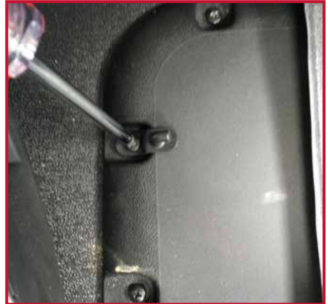
Figure 8 – Installation du crochet de retenue
