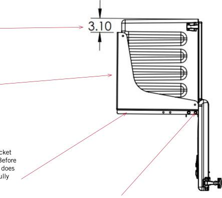
Allow clearance between the bracket assembly and the door when in the open position.
