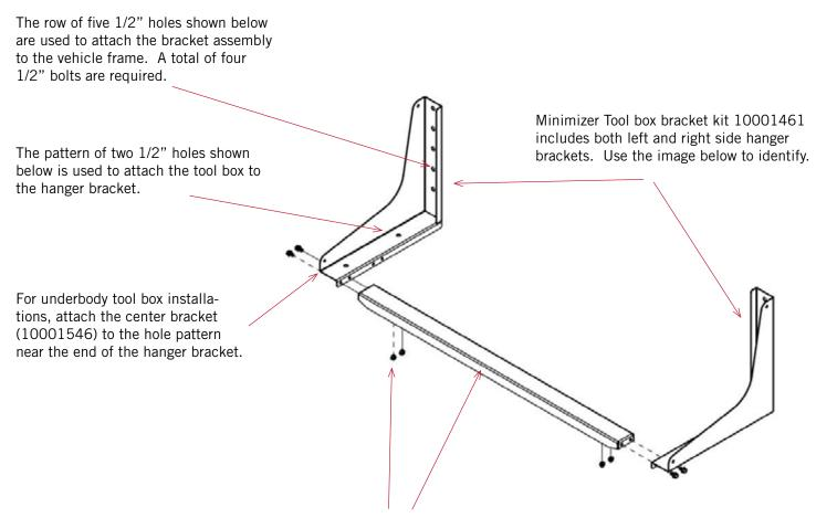
Attach center bracket (10001546) to the left and right hanger brackets. Use the set of 4 bolts and nuts from hardware kit 10001546 shown above.
