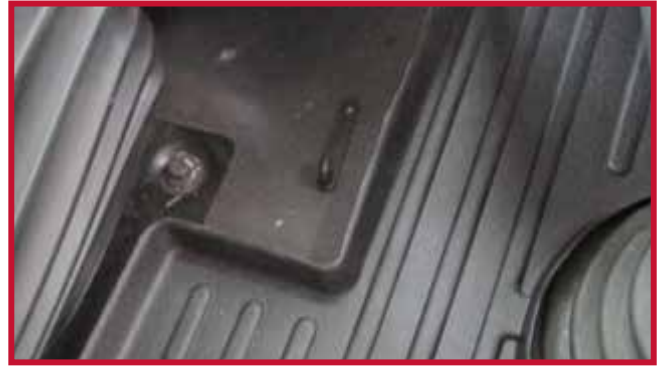
Figure 8 - Properly Installed Retention Hook
