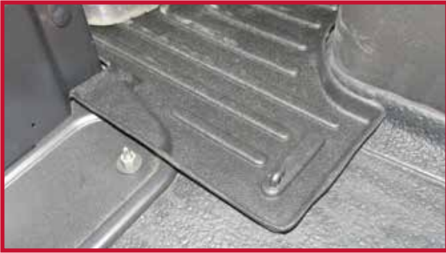
Figure 6 - Confirm Location Driver Mat and Hook
