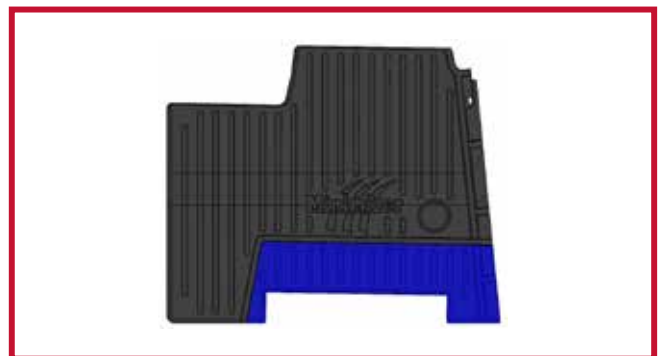
Figure 12 – Passenger Mat Trimming Diagram for kits 10002547, 10002551, 10002471 & 10002473
