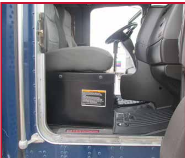
Figure 14 – Passenger Seat Battery Box with Trimmed Floor Mat
