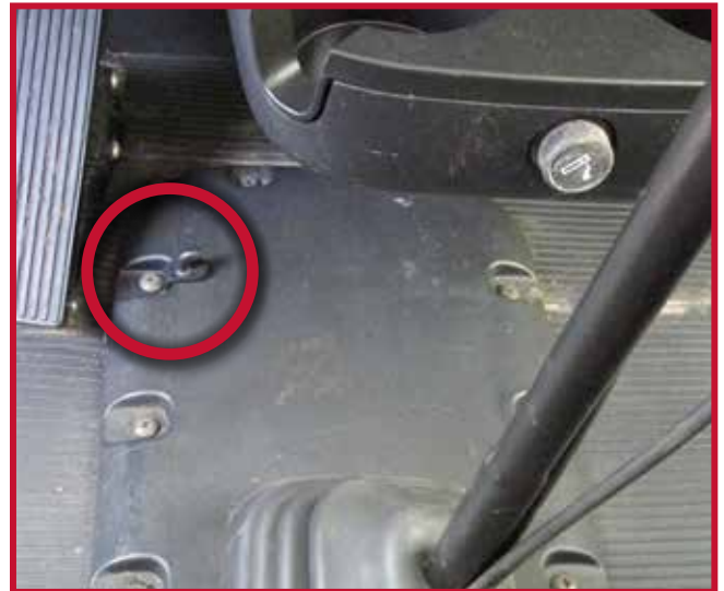
Figure 15 - Brake-Pedal Mounting Bolt
