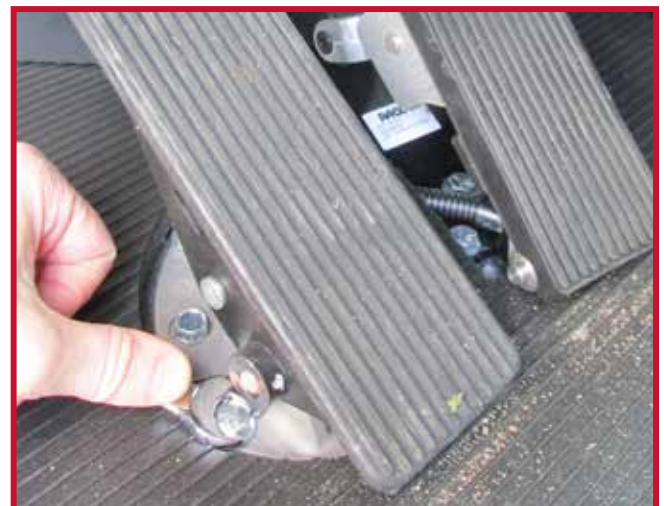
Figure 12 - Brake-Pedal Mounting Bolt
