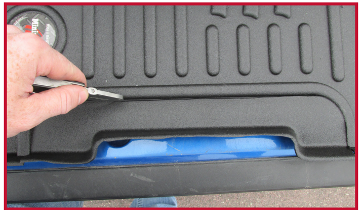
Figure 2 - Driver Mat Trim for Installation With Ezy Rider Seat or Aftermarket Seat.
