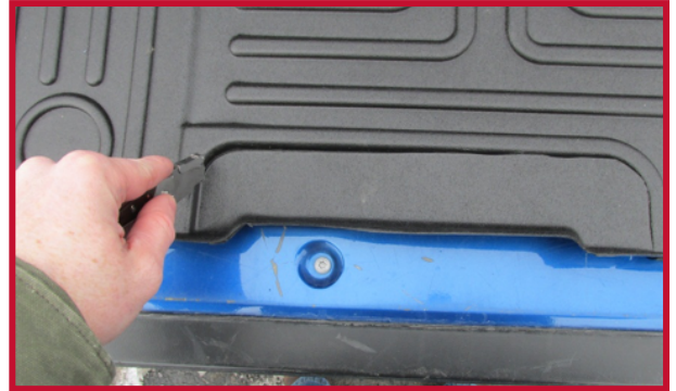
Figure 3 - Hand Trimming for Seat with Rubber Boot
