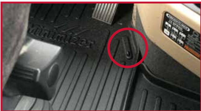
Figure 11 - Driver Mat Hook Installation
