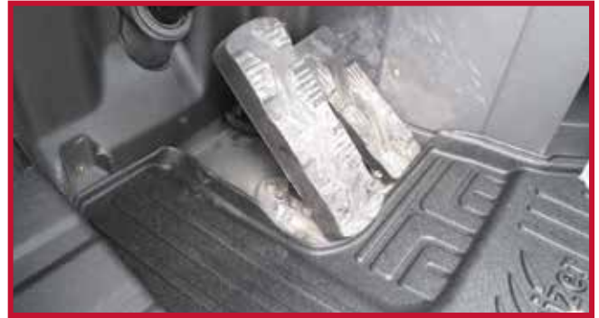
Figure 3 - Driver Mat Contact with Kick Panel
