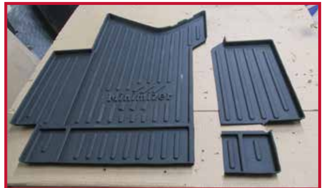
Figure 5 - Center Mat Trimming for Battery Box
