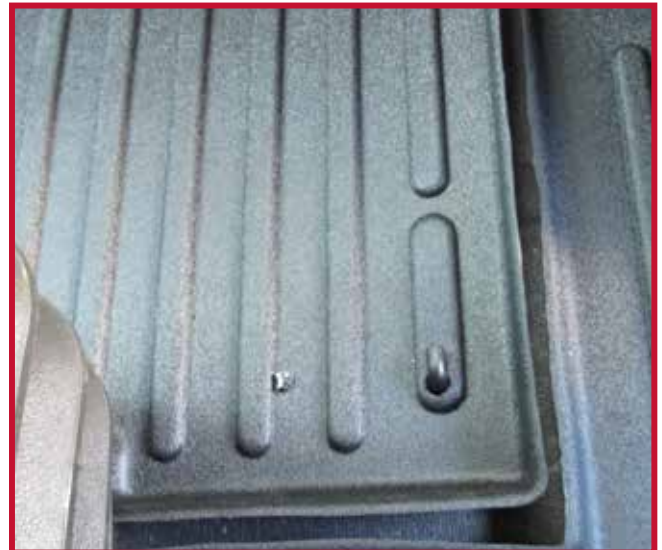
Figure 8 - Driver Mat Hook Installation
