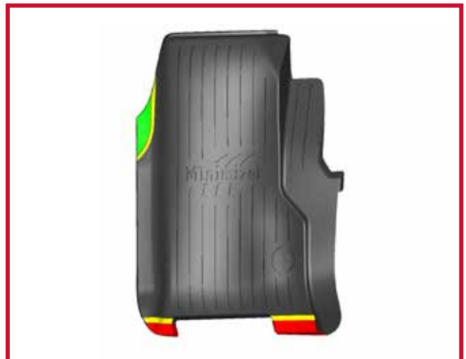
Figure 9 - Passenger Mat Trimming Diagram
