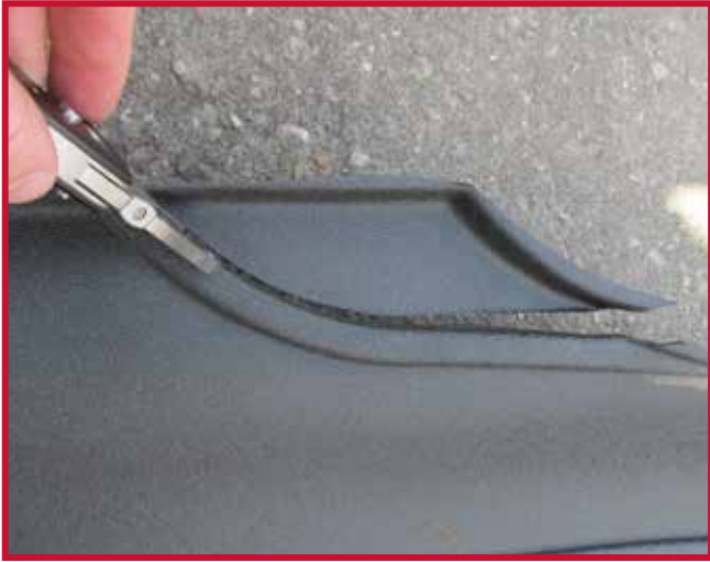
Figure 10 - Trimming Along Rib
