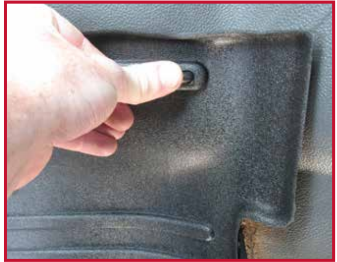
Figure 8 - Apply Pressure to Hook
