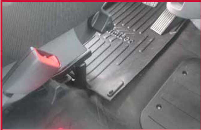
Figure 7 - Retention Hook Position
