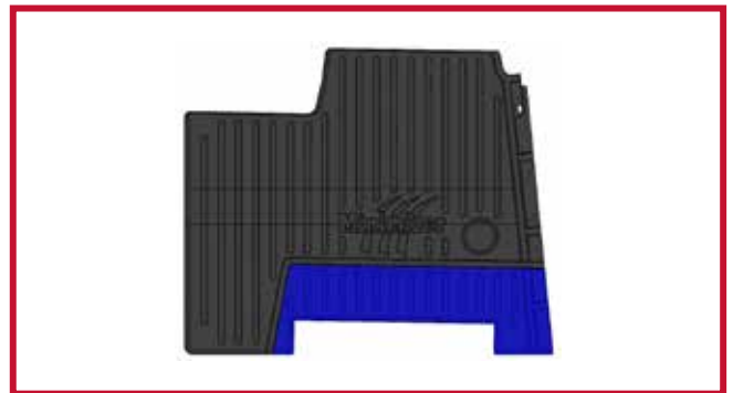
Figure 12 – Passenger Mat Trimming Diagram for kits 10002547, 10002551, 10002471 & 10002473
