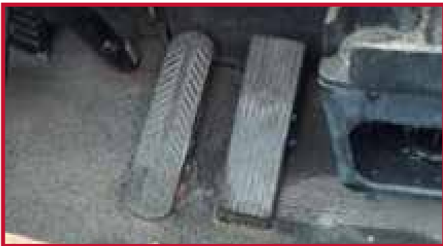
Figure 2 – Floor Mounted Throttle Pedal
