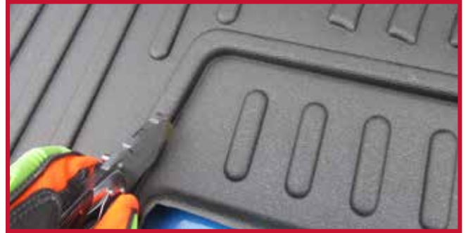
Figure 15 – Trimming Passenger Mat
