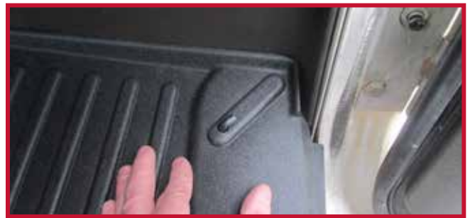
Figure 17 – Passenger Mat Hook Installed
