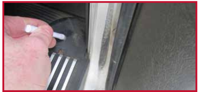
Figure 17 – Passenger Mat Hook Installed
