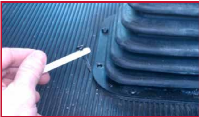
Figure 9 – Install Hook on Existing Screw
