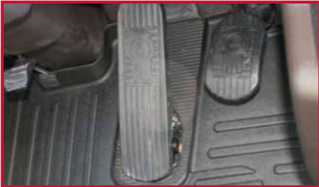
Figure 2 – Floor Mounted Throttle Pedal
