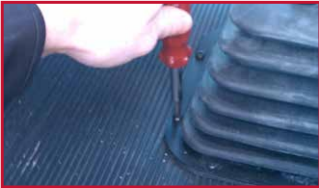
Figure 8 – Remove Screw from Shifter Boot
