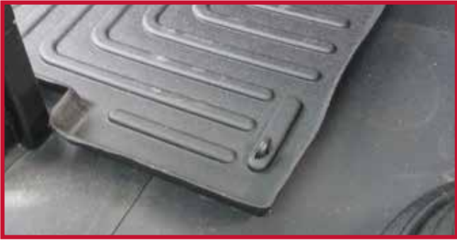
Figure 6 - Confirm Location Driver Mat and Hook
