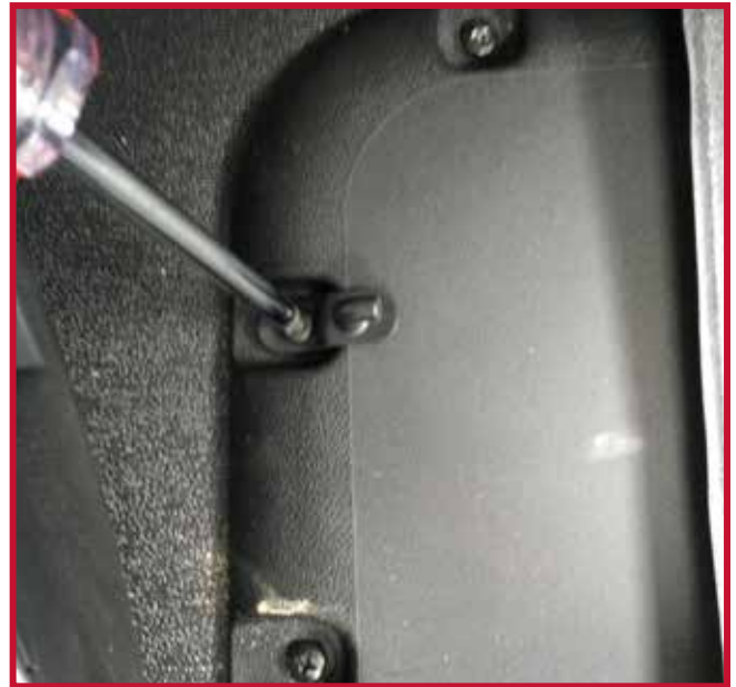
Figure 8 - Retention Hook Installation
