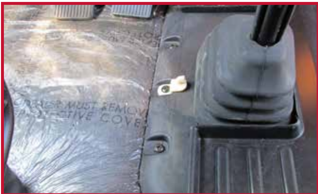
Figure 13 - Proper Hook Orientation
