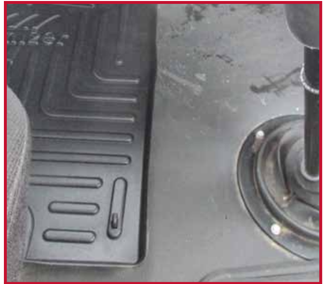
Figure 9 - Driver Mat Hook Installation
