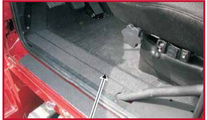
Figure 4 - Driver Side Electrical Tray
