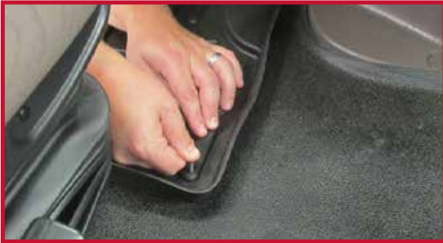
Figure 19 - Apply Pressure to Hook
