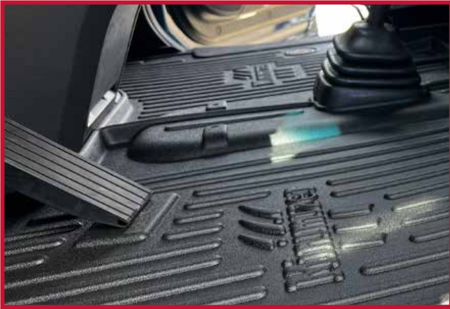
Figure 11 - Correct Floor Mat Position
