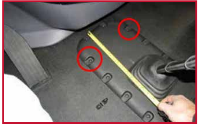
Figure 9 - Retention Hook Location
