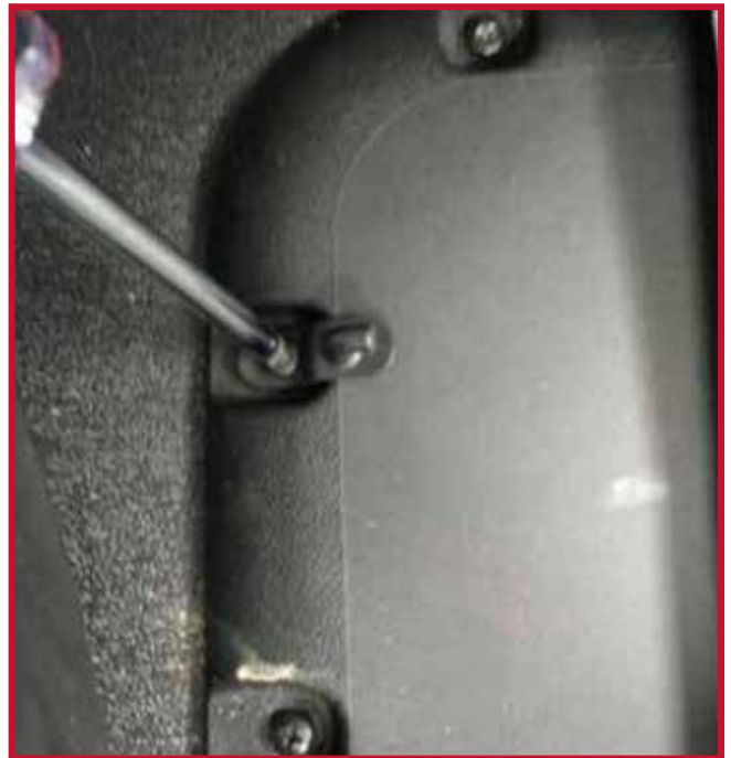
Figure 10 - Retention Hook Installation
