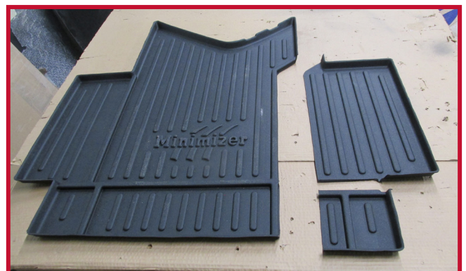
Figure 5 - Center Mat Trimming for Battery Box
