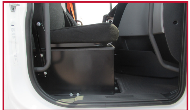
Figure 4 - Battery Box Passenger Seat
