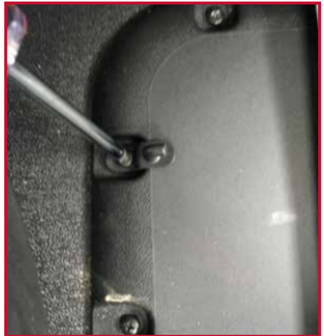
Figure 10 - Retention Hook Installation
