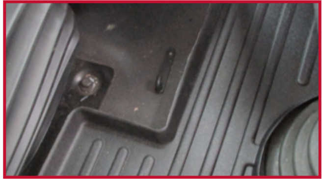
Figure 8 - Properly Installed Retention Hook
