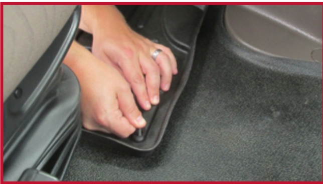
Figure 7 - Apply Pressure to Hook
