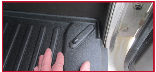
Figure 17 – Passenger Mat Hook Installed
