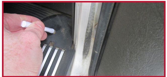
Figure 17 – Passenger Mat Hook Installed
