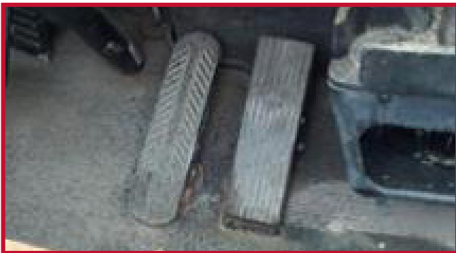
Figure 2 – Floor Mounted Throttle Pedal
