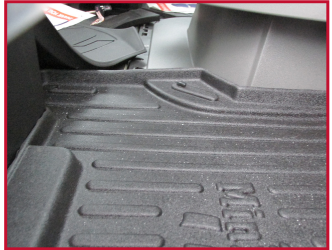
Figure 9 - Passenger Mat Retention Hook Location
